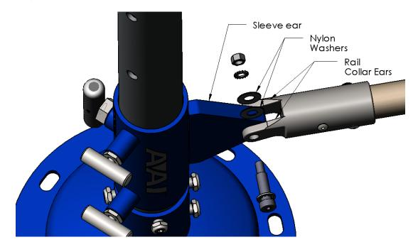
4. After adding the X rail your setup should look like the one shown below. Move the unit to the location where it will be installed. You will need sound and level concrete floor for proper installation of this system.
